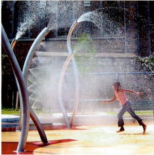
Ross Miller, Interactive Fountain , 2004, Sheehy Park, in Boston's Mission Hill neighborhood. Funded by the E. I. Browne Trust Fund of the City of Boston and coordinated by UrbanArts. The fountain conserves water because it is activated only by users. Seven remotely located motion sensors respond to people's presence and activity.
